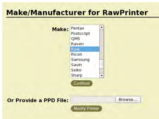
Figure 14-8. Setting the RawPrinter to be of Raw make
