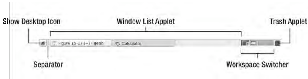
Figure 6-17. The Bottom Panel with applications
