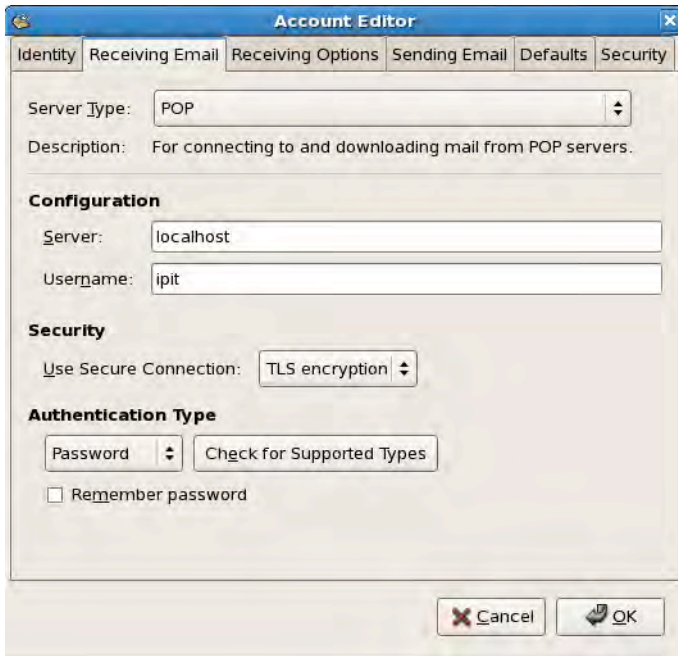
Figure 15-16. Adding security when downloading messages using OpenSSL
