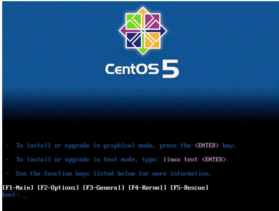
Figure 1-1. You have the option to install CentOS in graphical or text mode, or specify other options to troubleshoot the installation process or rescue an existing CentOS installation.
