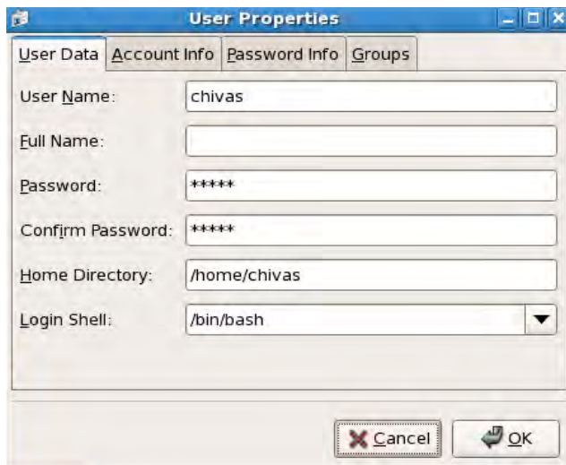
Figure 5-3. The User Properties dialog allows you to modify the account details of a user
