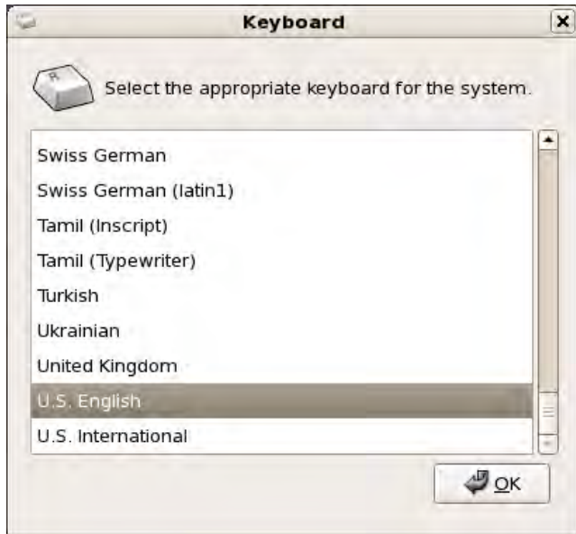
Figure 3-5. The system-config-keyboard program is used to change the keyboard layout.
